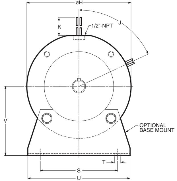
Note: Mounting base is optional and is ordered separately. Input Clutch (30) module and Output Clutch (40) are ordered separately.
