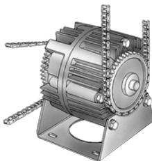
Electro Module assemblies may be mounted as separate drive units driven from the prime mover by V-belts, chain and sprockets, couplings, timing belts and other standard power transmission components.
